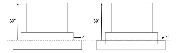
(c) Two-piece double die monuments - The base may be recessed 2" into a minimum 4" foundation; or secured upon the foundation with monument glue. Foundations must be installed flush with the grade of the ground and protrude 4" from all sides of the base.
