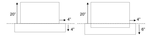
(b) Two-piece upright children's monuments - The base may be recessed 2" into a minimum 4" foundation; or secured upon the foundation with monument glue. Foundations must be installed flush with the grade of the ground and protrude 4" from all sides of the base.
