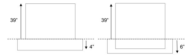
(b) Two-piece upright monuments - The base may be recessed 2" into a minimum 4" foundation; or secured upon the foundation with monument glue. Foundations must be installed flush with the grade of the ground and protrude 4" from all sides of the base.
